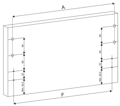
F = Internal cabinet width - 28mm A = Internal cabinet width - 24mm
