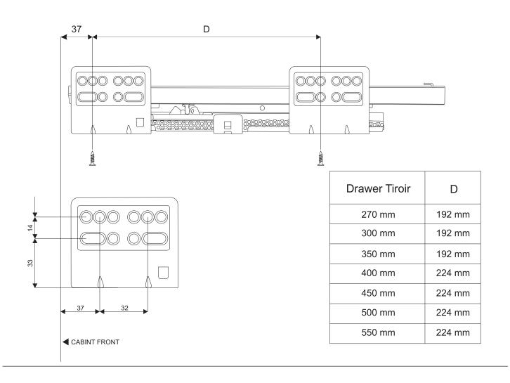
Assemble back connections to back panel.
