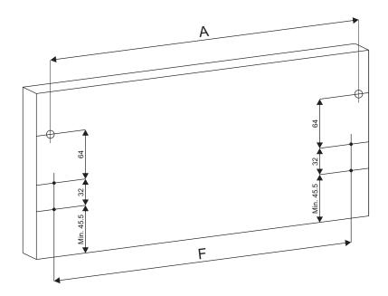
F = Internal cabinet width - 28mm A = Internal cabinet width - 24mm
