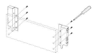
Assemble three drawer components by pressing the two sides against back panel.
